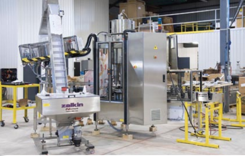
A Zalkin vertical conveyor and bottle capping system undergo testing at the Newmapak facility prior to being shipped and installed.
